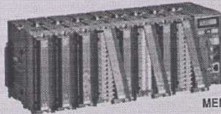
MEMORY HILOGGER LR8400-20 30 isolated analog input channels With built-in VOLTAGE/TEMP UNIT × 2 modules
